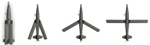
Upon deployment, AHM-1X opens wings to start the gliding descent to target.
